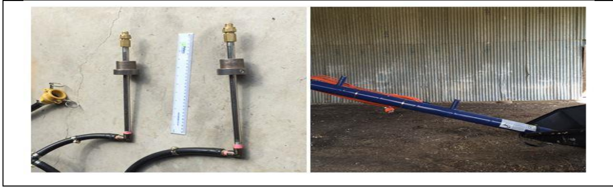
Fig.7. Spray application equipment designed for good coverage by applying treatment at two points in the auger
